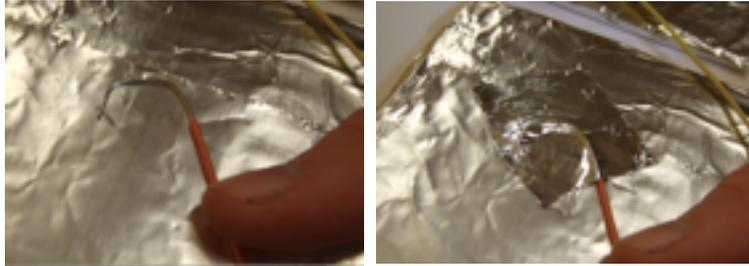
6. Twist the free ends of the wires together and solder them together
