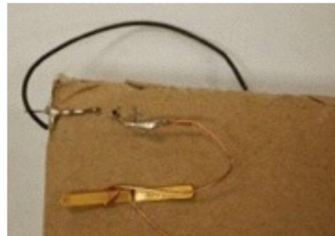
Twist the wire tightly around each brad to make sure the connection is tight.
